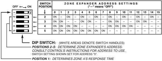
ON = NORMAL (300MS) RESPONSE, SHOWN (AS SHIPPED). OFF = FAST (10MS) RESPONSE TO AN OPEN.
