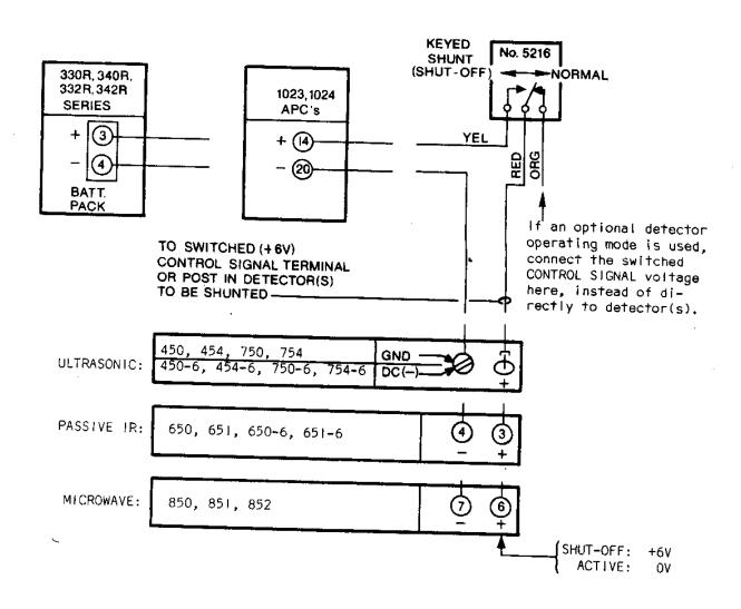
Diagram 3: TYPICAL CONNECTIONS, KEYED SHUNTING (SHUTOFF) OF SPACE PROTECTION DEVICES
