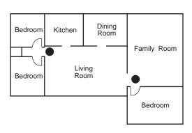
FIG. 2: In the family living units with more than one sleeping area, a smoke detector should be located to protect each sleeping area.
