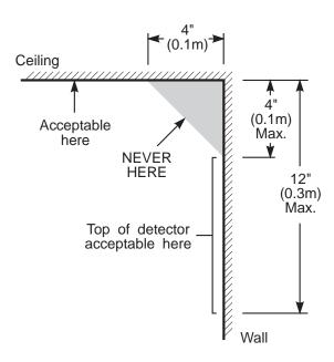
NOTE: Measurements shown are to the closest edge of the detector.
