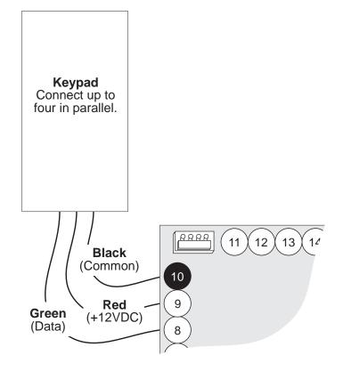
Figure 3: Keypad Wiring
