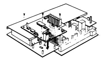
Install the 4152LMB by carefully inserting the square post connectors into the header. Take care not to insert the posts too far. Replace the lower circuit board cover.
