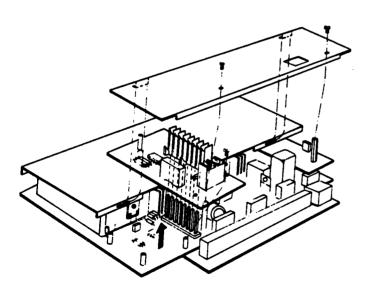
Remove the lower circuit board cover after removing the holding screws. Remove the No. 4153RD mounting screw. Carefully remove the 4153RD module from the square post connectors.
