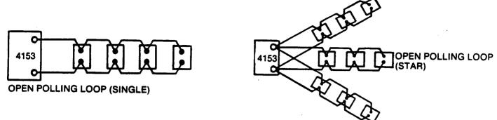
The following wiring configurations are used with the addition of the 4152LM.
