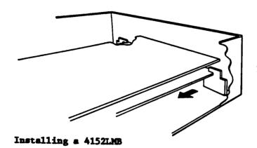
Remove the board by sliding it way from the slotted mounts.
