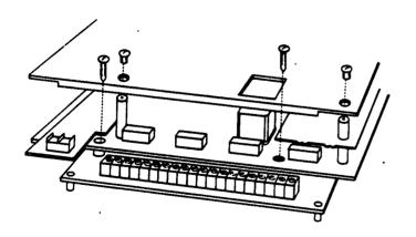
Remove lower cover and circuit board mounting screws.
