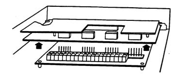
Lift and disconnect the circuit board from the square post connectors. Take care not to bend any of the connectors.
